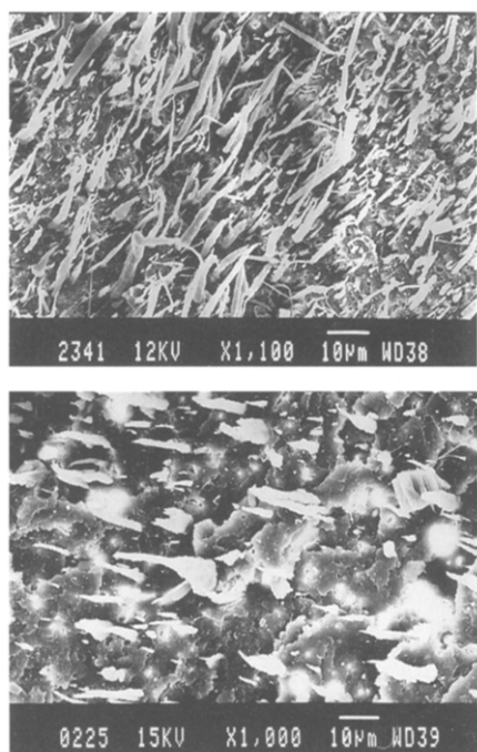
Figure 12 SEM micrograph of the PPESK/35%LCP blend extruded at a shear rate of (a) 250 \text{ s}^{-1} and (b) 14.4 \text{ s}^{-1}
